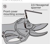
Secure the front cover with the front cover mounting screws (2 places). Tighten using the "2.5 hexagonal spanner for replacement blades".
