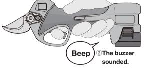
Quickly repeat the "pull and release" action of the trigger two or more times.
