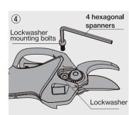
Turn the unit over and remove the lockwasher mounting bolt using the "4 hexagonal spanner for replacement blades" and remove the lockwasher.
