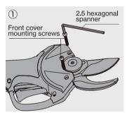
Using the "2.5 hexagonal spanner for replacement blades", remove the front cover mounting screws (2 places) from the front cover of the main unit housing. Be careful not to lose the screws.
