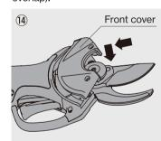
Place the front cover on the main unit housing. (Insert the claw into the main unit first, then push the front cover through).
