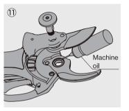
Overlap the upper blade and gear plate and insert the centre bolt. Apply 2-3 drops of machine oil to the sliding parts of the lower and upper blades (where they overlap).
