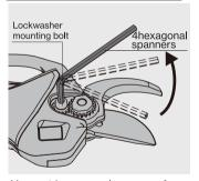
Use a 4 hexagonal spanner for replacement blades to loosen the lockwasher mounting bolt.
