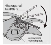
Tighten the lockwasher mounting bolt with a 4 hexagonal spanner for replacement blades.
