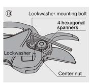
Place the lockwasher and lockwasher mounting bolt in the order shown in the illustration and tighten the lockwasher mounting bolt using the "4 hexagonal spanner for replacement blades" to secure the lockwasher.
