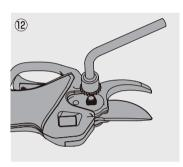
Turn the unit over while supporting the rear bolts by hand to prevent them from falling out, then tighten the center nut with a "13 box spanner for replacement blades".
