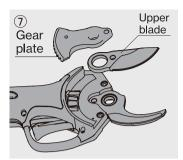
Remove the gear plate and top by hand.
