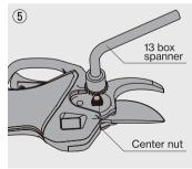
Remove the center nut with the "13 box spanner for replacement blades".
